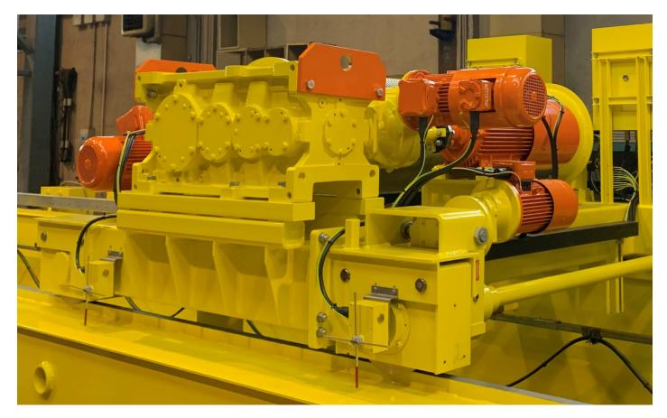
ARG Series rope winches set a benchmark in lifting equipment, thanks to a unique configuration in the world of lifting appliances, using lifting gears with differential unit, combined with the latest technology in motors and controls.
